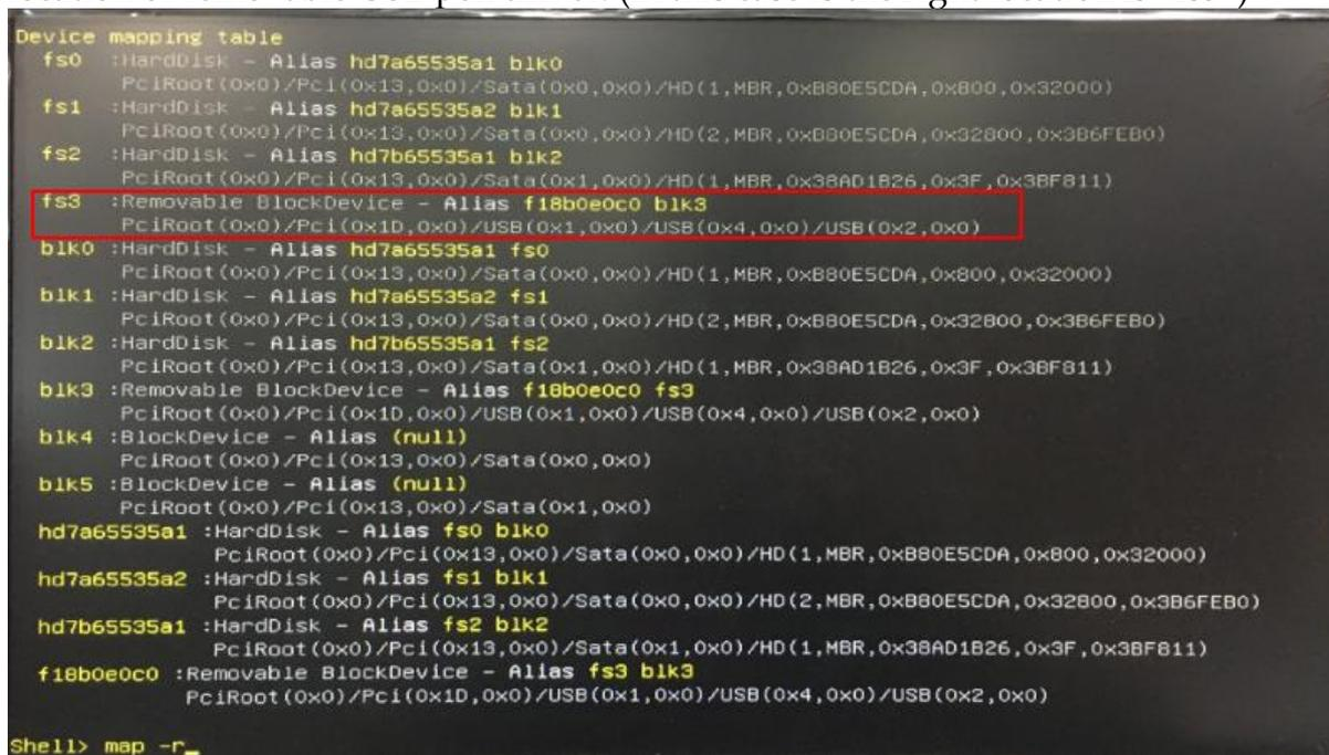
Step5. Type “fs3:” command to switch to the root of the USB pen drive. And type “dir” to find the directory of fs3.
