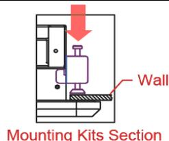
2. Screw the Clip tightly (Torque Value = 8kg )
