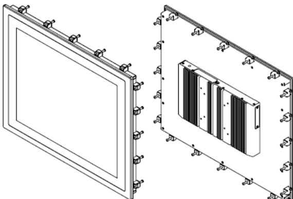
3. Hook the mounting clamps with screws (included) from the back side
