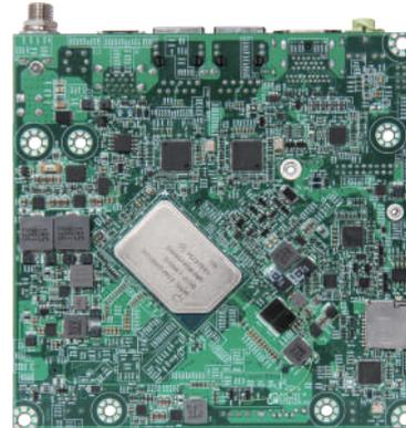
NANO-6063 is based on Intel® Atom® Elkhart Lake family processor. This processor not only supports the range of industrial temperature standard which is from -40°C to 85°C but operates in certain 12W with low-power consumption. Succeeding previous version, NANO-6062, the flexibility of systematic expansions is suitable for Medical, Panel PC and Kiosk. To support Intel® I225 Gigabit Ethernet is fit in Industrial Automation, and Digital Signage application.
