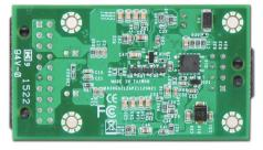
GADIWA-B1120 is a DC to DC 12V input board type converter. It normally support continuous 120 Watts and peak 160 Watts.
